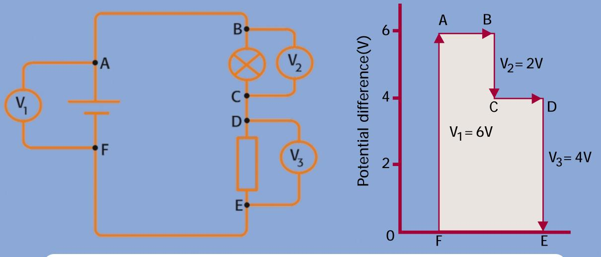
The total voltage across the circuit components equals the battery voltage
